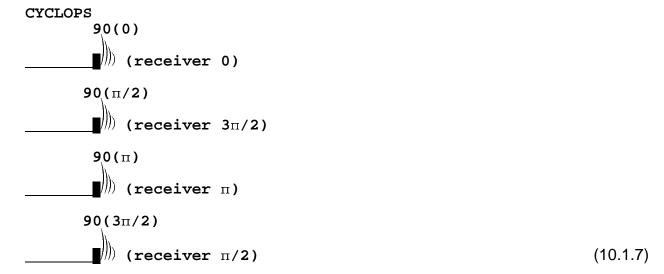
The sequences in 10.1.7 are a schematic of the CYCLOPS phase cycle procedure. In the following sections, we will analyze this procedure in detail, but we first must discuss an implementation of the product operators that is convenient for the discussion of phase cycling.
