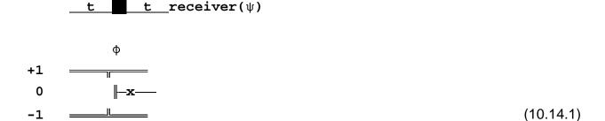
In this sequence,  $I^+$  coherence is transferred to  $I^-$  and vice versa by the 180° pulse. As described in Section 10.10, an imperfect pulse will transfer some  $I^+$  to  $I_z$ , which may cause artifacts in the final spectrum. EXORCYCLE removes the  $I_z$  component by shifting the phase of the 180° pulse and thus the phase of the coherence.
