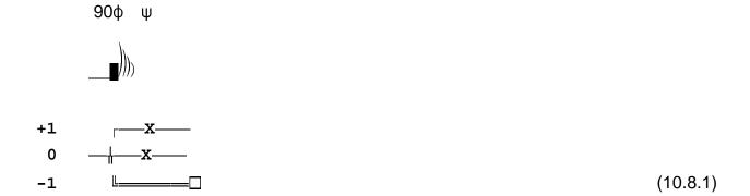
In sequence 10.8.1, a single 90° pulse excites Z magnetization at coherence order 0 to orders ±1. To eliminate quadrature images +1 coherence must be blocked. Removal of systematic noise is accomplished by blocking 0 order coherence.
