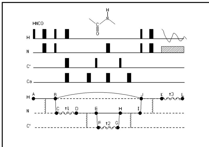
**Figure 14.1.** Pulse Sequence and CFN for the three dimensional HNC(O) experiment.
