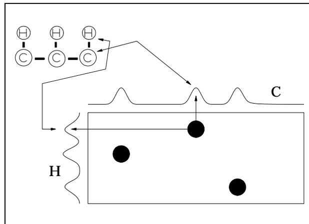
**Figure 15.1.4.** Schematic  $^{13}\text{C}\{^1\text{H}\}$  heteronuclear chemical shift correlation spectrum.
