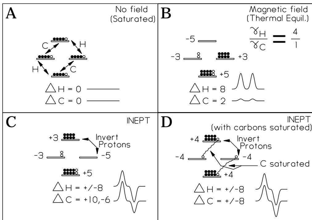
**Figure 15.1.2.** Energy level diagrams of a two-spin  $^1\text{H}-^{13}\text{C}$  system showing various polarizations.
