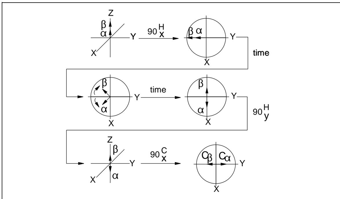
**Figure 15.1.1.** Vector representation of INEPT transfer for a coupled  $^1\text{H}$ - $^{13}\text{C}$  spin system.
