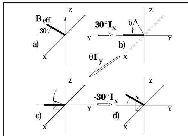
**Figure 6.4.** Rotation of  $I_z$  magnetization about a tilted effective field,  $\mathbf{B}_{\text{eff}}$ .
