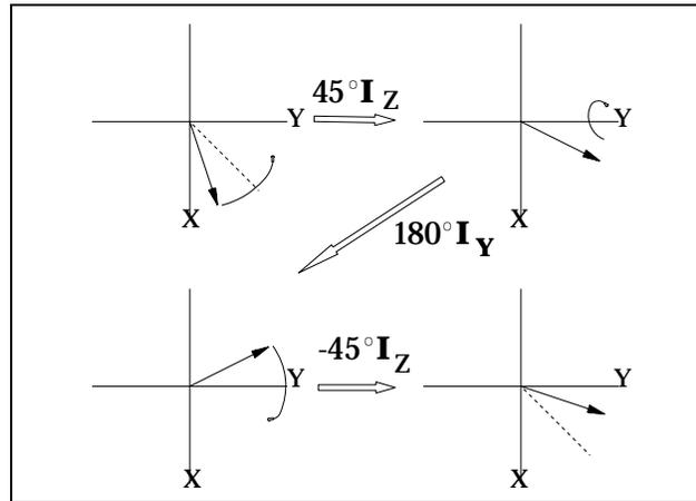
**Figure 6.6**  $180^\circ$  rotation of a vector in the XY plane about an axis phase shifted  $45^\circ$  away from the X axis.
