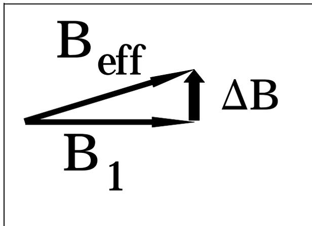
**Figure 6.2.** Vector addition of the residual static field,  $\Delta B$ , and the applied RF magnetic field,  $B_1$ , to give an effective field,  $B_{eff}$ .
