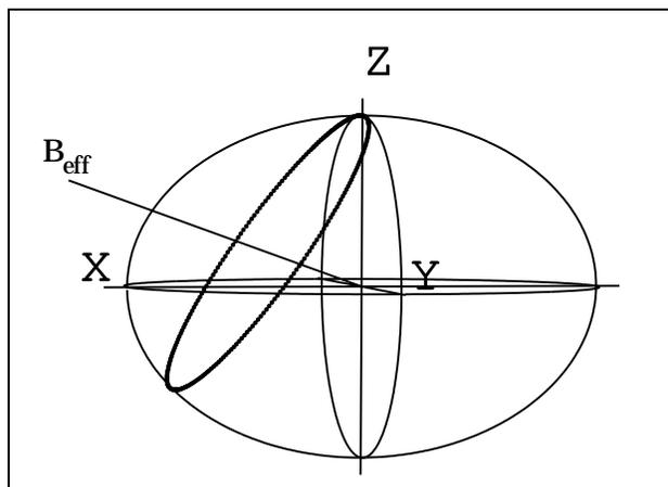
**Figure 6.3.** Trajectory of tip of a spin vector around a tilted  $B_{eff}$ .
