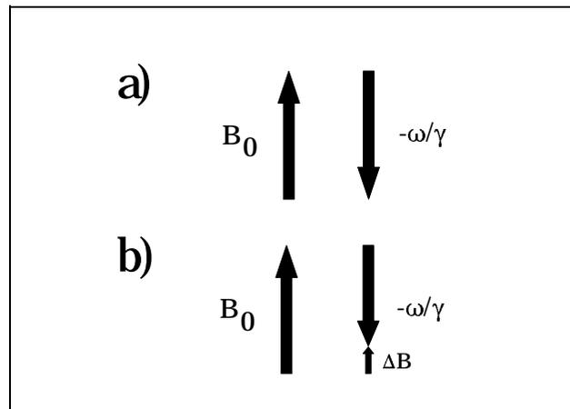
**Figure 6.1.** Fictitious field,  $-\omega/\gamma$ , opposing the static field,  $\mathbf{B}_0$ . a) If the spin is on resonance, then  $\Delta B=0$ . b) For spins not on resonance then there is a residual field,  $\Delta B$ .
